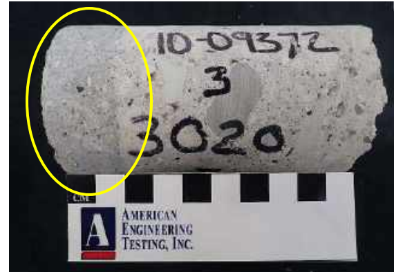
Figure 3 – Overall profile of Core 3 (north end of deck) from the petrographic analysis for concrete testing.
